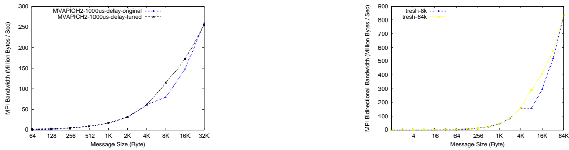
Figure 9. MPI-level throughput using MVAPICH2 with varying protocol thresholds for 1ms delay: (a) Bandwidth (b) Bidirectional Bandwidth
