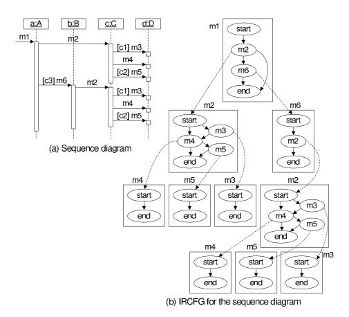
Fig. 1. Sample sequence diagram and the corresponding IRCFG.
