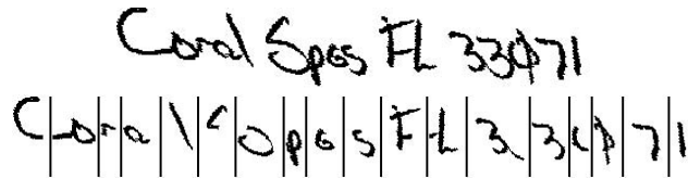
Figure 6.1: Example of a city-state-zip image (a) The line containing the city name ( Coral Spgs ), state name ( FL ) and zip code ( 33071 ). (b) Results of segmentation.
