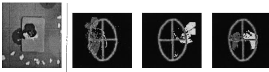
Figure 10. These images show the motion energy that is detected from the overhead camera when a person is “rowing” as they sit on top of the bed. The ellipse represents the position and orientation of the bed, extracted by the system; the colored pixels indicate where the system detected motion. The left, middle, and right images show rowing on the left, right, and both sides of the boat, respectively. The amount of movement at any time is compared with the maximum movement detected so far to compute how vigorously people are rowing and on which side of the bed.
