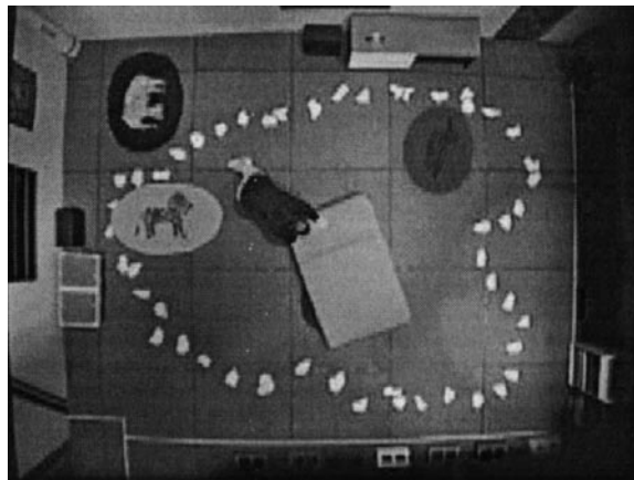
Figure 2. The KidsRoom is furnished like a real children's room, complete with furniture, decorations, and a movable bed. Rugs and stone-like markers are used throughout the narrative. Four speakers project sound into the space. Colored cinder blocks at the base of the large projection screens protect the screens (which comprise the right and bottom walls in this image) from the movable bed. The square on the floor in the bottom left marks the "door," through which people enter and exit the space.
