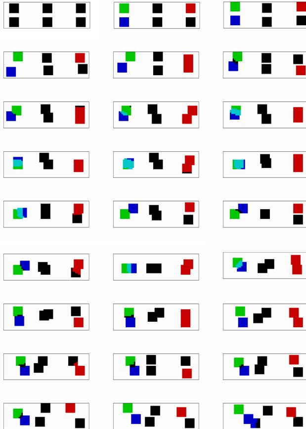
Figure 6: Multiple object tracking. Processing an image with three targets and three distractors. Each pixel is painted in red, green, blue, or a mixture of these colors. A pixel is red/green/blue if a “red”/“green”/“blue” oscillator in the column that corresponds to this pixel is in the resonant state. A pixel is cyan if both oscillators in the “blue” and “green” layers are in the resonant state. A pixel is black if no oscillator in the column is in the resonant state. A pixel is white if it belongs to the background.
