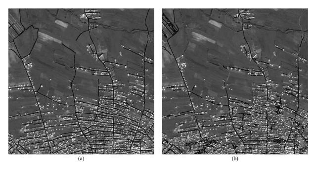
Fig. 11. Road extraction from Ikonos1-Sub1. (a) Red band image of Ikonos1-Sub1 with reference road data marked. (b) Extraction result using the proposed method with the parameters  $W_z = 60$ ,  $\theta_p = 35$ ,  $N_p = 40$ , and  $W_{zq} = 0.85$ .
