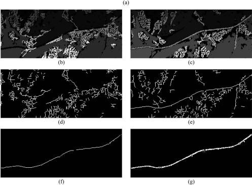
Fig. 8. Road extraction from a satellite image. (a) Satellite image containing a road with  $300 \times 120$  pixels. (b) LEGION segmentation result with bright road thresholding. (c) LEGION segmentation result with dark road thresholding. (d) Candidate medial axis points in (b). (e) Candidate medial axis points in (c). (f) Grouped medial axis points based on (e). (g) Road extraction result. The parameters used here are  $W_z = 60$ ,  $\theta_p = 45$ ,  $N_p = 50$ , and  $W_{zg} = 0.85$ .
