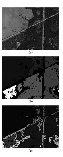
Fig. 4. LEGION image segmentation. (a) Satellite image containing roads. (b) Result of LEGION segmentation where each gray level indicates a distinct segment. (c) Result after the step of obtaining road segments.
