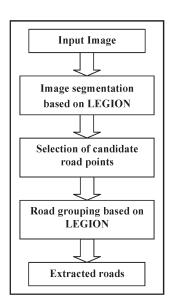
Fig. 3. Flow diagram of the proposed system for automatic road extraction.
