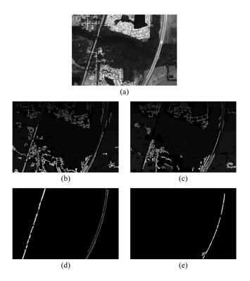
Fig. 9. Road extraction from another satellite image. (a) Satellite image containing two main roads with 300 × 200 pixels. (b) LEGION segmentation result with bright road thresholding. (c) LEGION segmentation result with dark road thresholding. (d) Road extraction result based on (b). (e) Road extraction result based on (c). The parameters used here are  $W_z = 40$ ,  $\theta_p = 55$ ,  $N_p = 60$ , and  $W_{zg} = 0.85$ .
