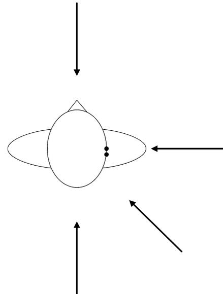
Fig. 11. Room configuration. The HATS (seen from above) is placed in the middle of a room with a reverberation time of 400 ms. The two-microphone array is placed at the right ear. The distance between the microphones is 12 mm. The four sources arrive from positions of 0°, 90°, 135°, and 180°. The distance from the center of the head to each of the loudspeakers is 2 m. The room dimensions are 5.2 × 7.9 × 3.5 m.
