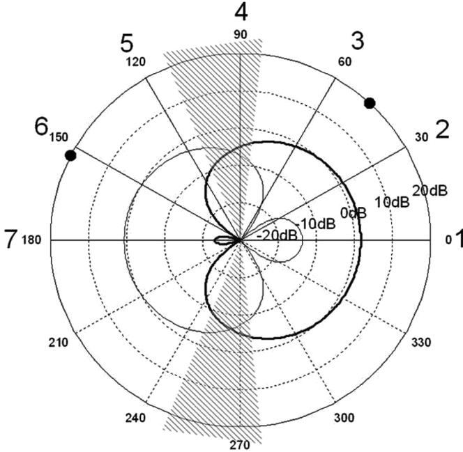
Fig. 7. As in Fig. 2, the polar plots show the gain for different directions. Comparison between the gains determines the binary masks. Within the shaded areas, the gain is almost equal. Source signals that arrive from a direction close to where the gains are almost equal will (depending on the parameter  $\tau$ ) either exist in both masked signals or in none of the masked signals. Therefore, the algorithm may fail to segregate such source signals from the mixture.
