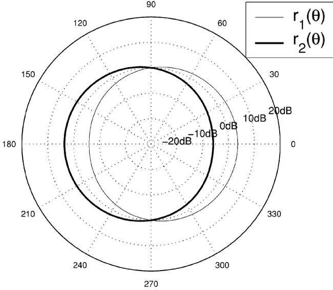
Fig. 1. Two directional microphone responses are shown as a function of the direction  $\theta$ .
