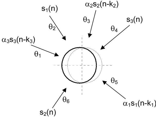
Fig. 8. Simple reverberant environment with three sources each having one reflection. As in Fig. 1, the impinging signals are recorded by a two-microphone array with directional responses, so that each direction corresponds to a certain set of directional microphone responses. Here, each reflection can be regarded as a single source impinging the microphone array.
