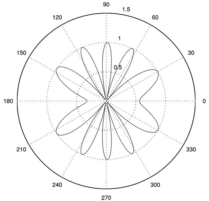
Fig. 12. Typical HF microphone response. The response is given for the frequency of 4000 Hz and a distance of 20 cm between the microphones. The half-wavelength at 4000 Hz is  $\lambda/2 = 4.25$  cm. Since four whole half-wavelengths fit between the microphones, four nulls appear in the interval  $0^\circ \leq \theta \leq 180^\circ$ . Such a beam pattern cannot efficiently be used to estimate the binary mask.
