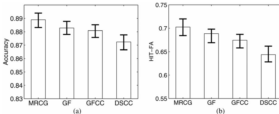
Fig. 6. Median value and interquartile range of 50 test sentences for average performance on six noises. Results are shown for top four features in terms of classification accuracy and HIT-FA rate (a) Accuracy (b) HIT-FA.
