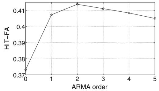
Fig. 4. Effect of the ARMA post-processing order for the PLP feature with babble noise at  $-5$  dB SNR.
