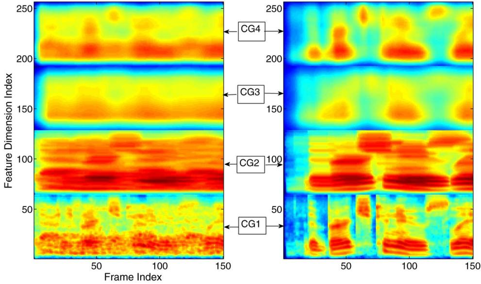
Fig. 3. (Color online) Visualization of the MRCG feature. Left side shows MRCG features extracted from a mixture, while the right side shows MRCG features extracted from premixed clean speech. In CG2-4, feature patterns of the mixture resemble the ones of clean speech to some extent, indicating the MRCG feature could partially retain spectrotemporal patterns of speech in the presence of noise.
