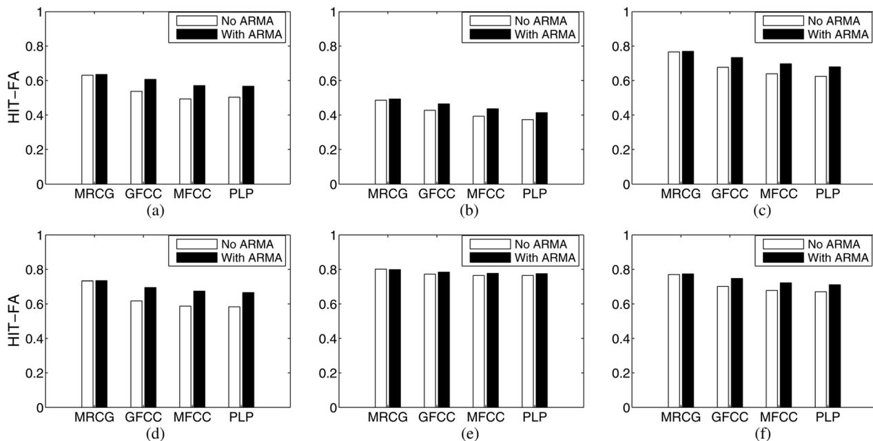
Fig. 5. Effects of ARMA filtering in terms of HIT-FA rate (a) Factory (b) Babble (c) Engine (d) Cockpit (e) Vehicle (f) Tank.
