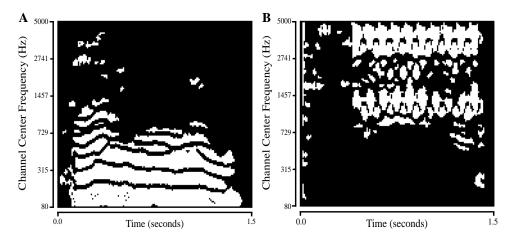
Figure 3: A. Snapshot showing the activity of the second layer shortly after the start of simulation. Active oscillators (white pixels) correspond to the speech stream. B. Another snapshot, taken shortly after A. Active oscillators correspond to the telephone stream.
