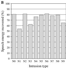
Figure 4: A. SNR before (black bar) and after (grey bar) separation by the model. Results are shown for voiced speech mixed with ten intrusions (N0 = 1 kHz tone; N1 = random noise; N2 = noise bursts; N3 = 'cocktail party' noise; N4 = rock music; N5 = siren; N6 = trill telephone; N7 = female speech; N8 = male speech; N9 = female speech). B. Percentage of speech energy recovered from each mixture after separation by the model.
