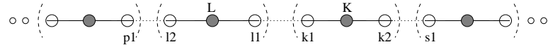
Figure 1.1: Each pair of brackets constitutes one cluster of unit radius, and shaded nodes denote cluster leaders.
