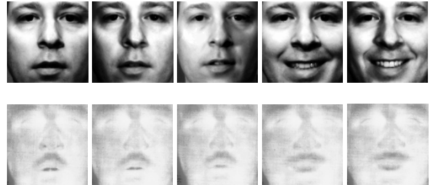
Figure 3: The normalized faces: visual (top row) and thermal (bottom row) images of the same individuals taken from different conditions
