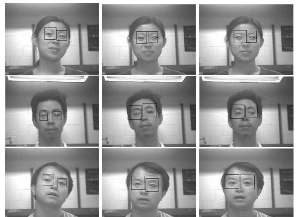
Figure 3. The result of using the difference image and a cascaded classifier for eye detection.
