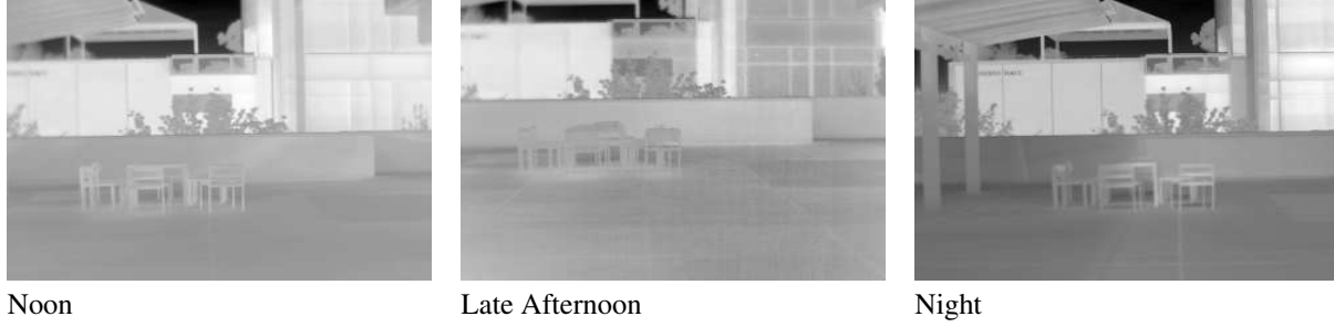
Figure 4. Thermal images of the background at different time in a day recorded from the thermal infrared sensor: noon, late afternoon and night, each of which is normalized by the temperature range individually.
