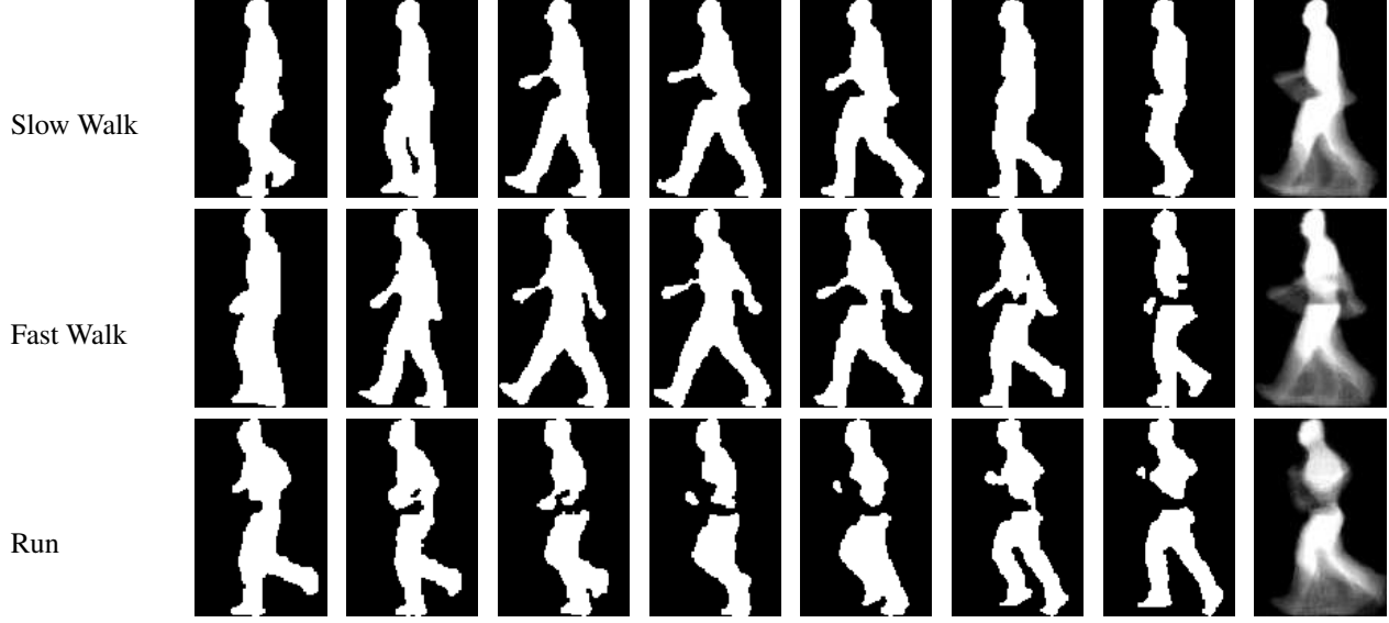
Figure 3. Examples of normalized and aligned silhouette frames in different human motion sequences. The rightmost image in each row is the corresponding gait energy image (GEI).
