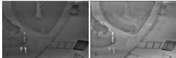
Figure 6: Extracted background using 24 frames in #8 only (left) and 48 frames in #8, #10 together (right).
