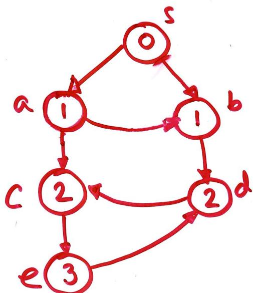
For  $u \in V$  define  $\delta(s, u)$  as the number of edges of a shortest path from  $s$  to  $u$ .
