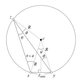
Figure 1.18: Relationships between the circumradius *R*, shortest edge  $\ell_{\min}$ , and smallest angle  $\theta$ .
