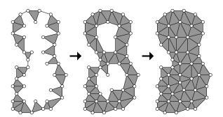
Figure 1.7: Advancing front mesh generation.
