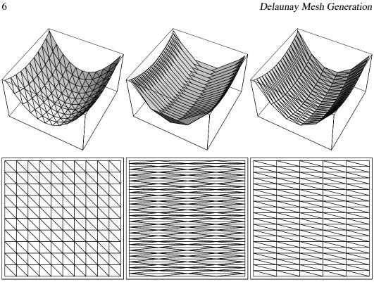
Figure 1.3: An illustration of how large angles, but not small angles, can ruin the interpolated gradients. Each triangulation uses 200 triangles to render a paraboloid.
