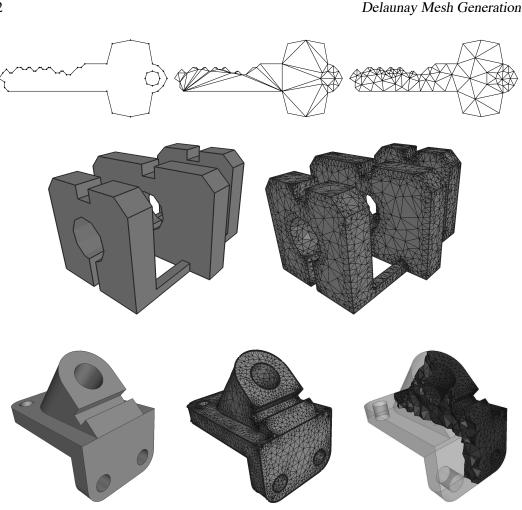
Figure 1.1: Finite element meshes of a polygonal, a polyhedral, and a curved domain. One mesh of the key has poorly shaped triangles and no Steiner points; the other has Steiner points and all angles between 30° and 120°. The cutaway view at lower right reveals some of the tetrahedral elements inside the mesh.
