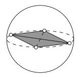
Figure 1.9: The mesh generator's nemesis: a sliver tetrahedron.
